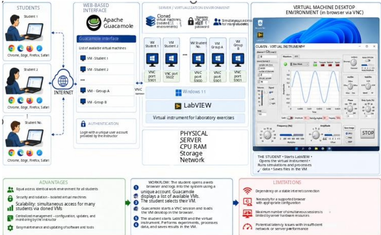
Figure 3.79. Block diagram of the remote access to the virtual laboratory environment
