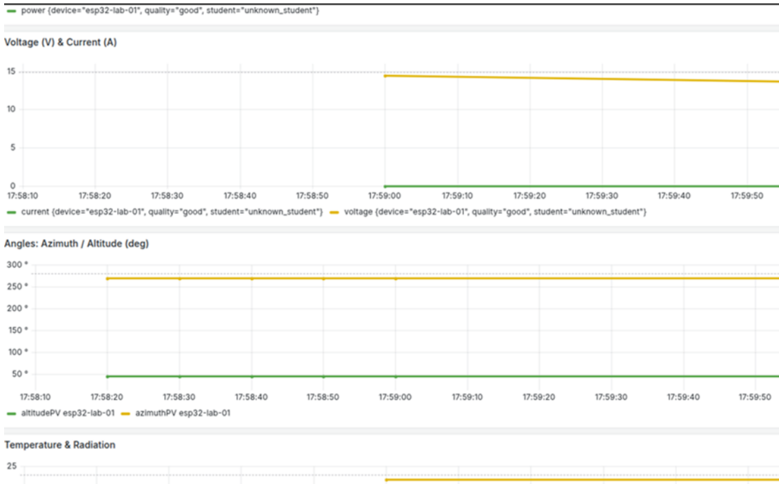
Fig. 4.19. Dashboard in Grafana for visualization of telemetry data from the photovoltaic system stored in InfluxDB
