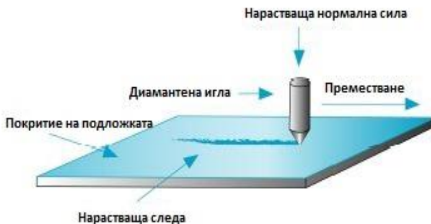
Fig.3.10. How the scratch test works [127, 136]
