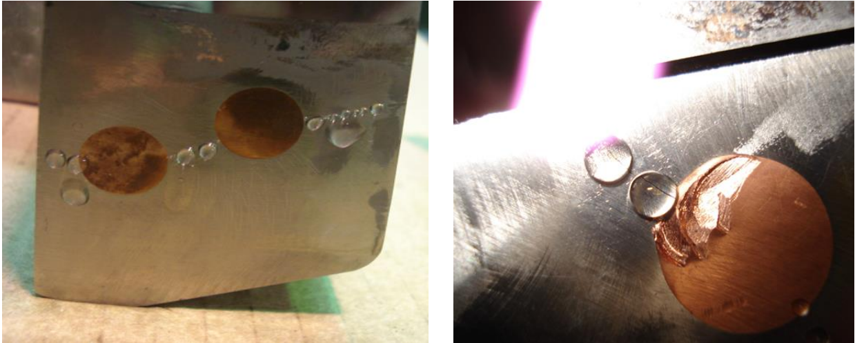
Fig.6.1. Leakage from the cooling circuits due to cracks in the area of the plugs
