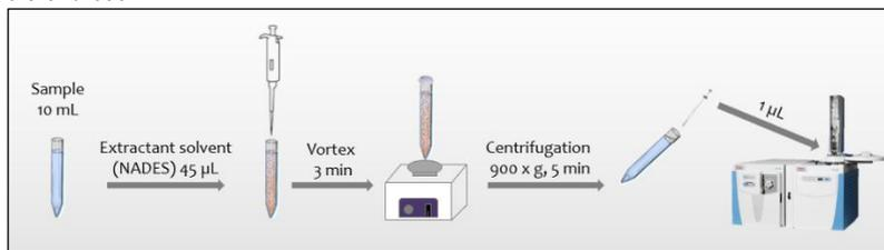
**Figure 2:** NADES-based-DLLME-GC-MS/MS procedure for pesticide analysis.
