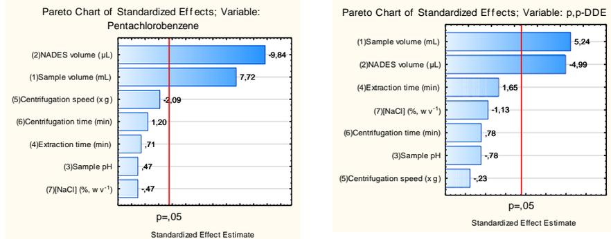
**Figure 11:** Pareto charts of standardised effects from Plackett-Burman design for the studied target analytes.
