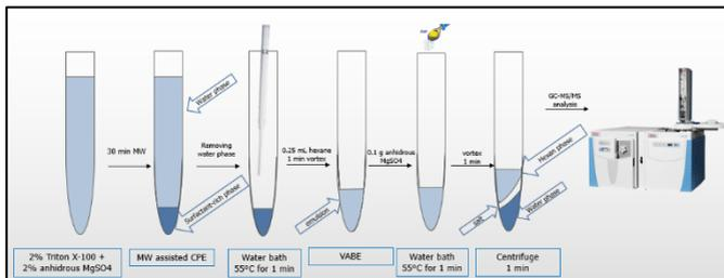
**Figure 1:** MW-CPE-GC-MS/MS procedure for pesticide analysis.
