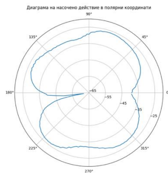
Figure 6.10. Radiation pattern in polar coordinates
