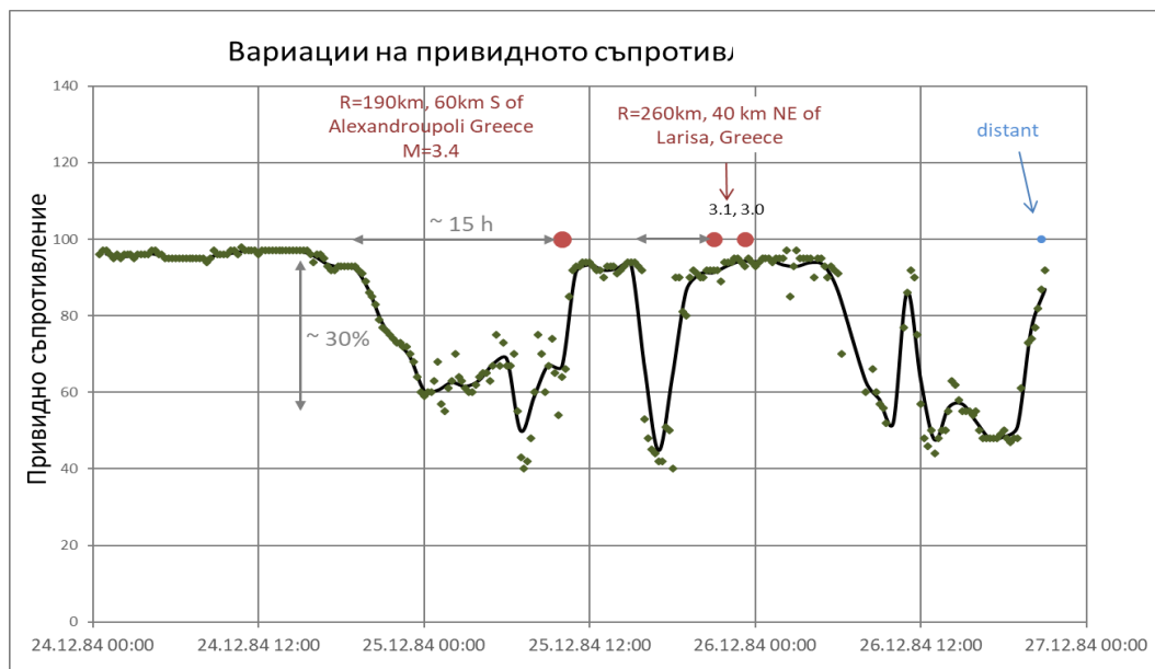
Fig. 1.23. Variations of apparent resistivity recorded by the author in the area of NAO "Rozhen"
